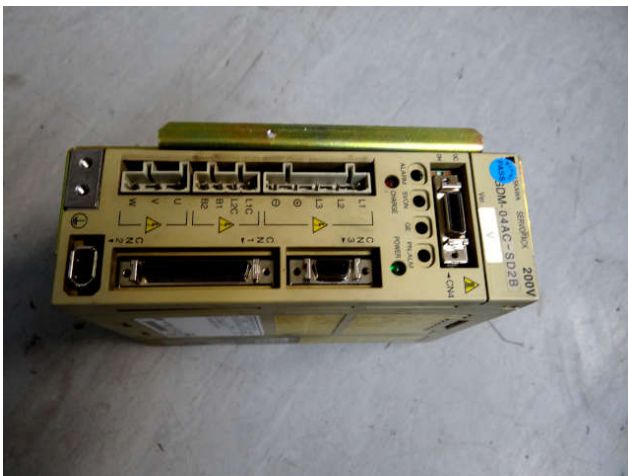
Servopack before repair
