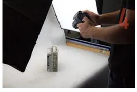
We take pictures of the device and the parameters and jumpers. Further customer wishes and description of defect are considered and documented.
